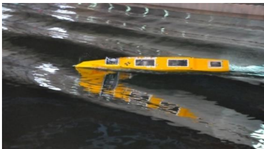
Fig.3: The free-running experiment of broaching with the tumblehome in CSSRC
