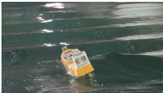
Fig.4: The free-running experiment of pure loss of stability with the tumblehome in CSSRC
