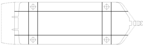
Figure 5: Main constructional bulkheads of a WTI jack-up.
